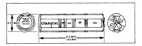
PROPELLING CHARGE M1. This is a "green bag" charge divided into a base and four increments for firing in zones 1 thru 5. The increment bags are tied together by cloth tying straps. An igniter charge in a red
